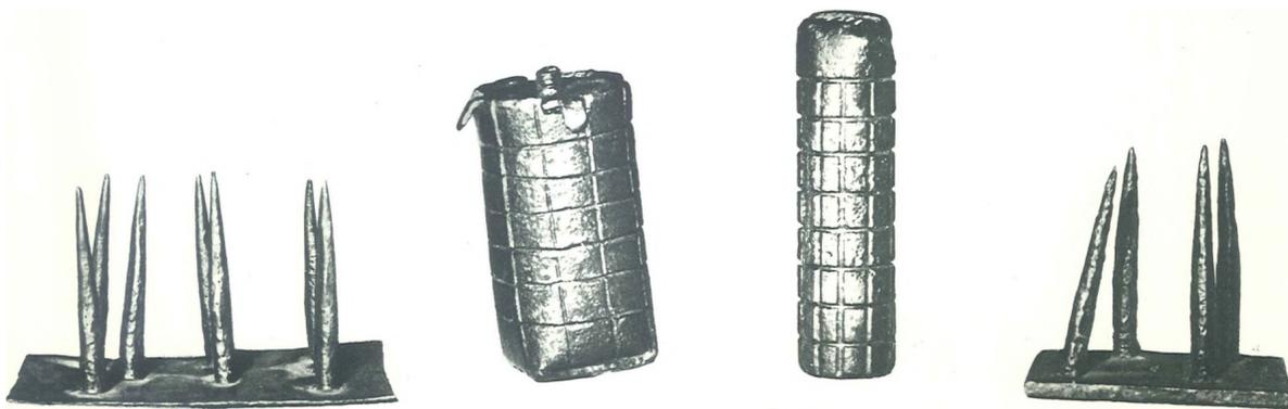
243. PROJEKTI PARTIZANSKIH RADIONICA NOP ODREDA U BOSNI : BOMBE IZRADIVANE OD VODOVODNIH CEVI I SILICI ZA DIVERZIJE NA OKUPATOROVU MOTORIZACIJU, RAĐENO I UI-OIREELJAVANO U USTANKU 1941. GODINE
